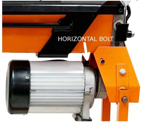
Remove the complete motor and pump bracket assembly. There are two O-rings in holes in the face of the pump bracket, ensure you do not lose these.
