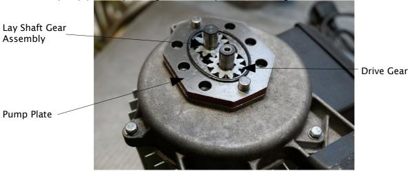
Remove the small pin (part 70) that keys the drive gear to the motor shaft. Do not misplace this as the pump will not drive without it.
