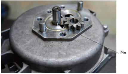
Undo the three long bolts holding the end cover to the motor and remove the end cover. Note that if you have not removed the small pin (70) then you cannot draw the shaft through the cover.
