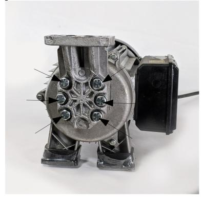
Remove the pump plate, lay shaft gear assembly and the drive gear from the motor shaft.
