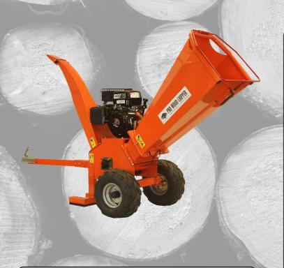
The FM13WC is a large, tow-able wood chipper ideal for domestic or commercial use. It has a 13hp engine which is capable of shredding branches up to a diameter of 100mm (4 inch). It is powered by the latest generation LCT Maxx Series 414cc 13hp 4 stroke engine. An attachable tow bar and safety chain allows the chipper to be towed at a max speed of 5mph off-road for use on fields and farms etc.
