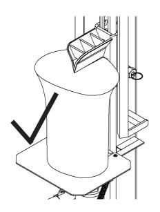
If splitting a log of extremely irregular shape, e.g. where one end flares considerably in diameter. Place the log so the widest end is uppermost.
