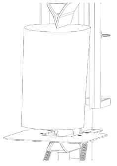
Use the left pedal to gently raise the lower blade and lift the log, this will in turn lift the upper blade. Continue raising the log until the locking pins on the upper blade are heard to click into place in the next set of holes.
