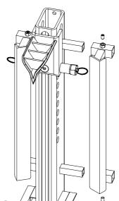
Remove the two grub screws and slide the log rail off the mounting tubes.
