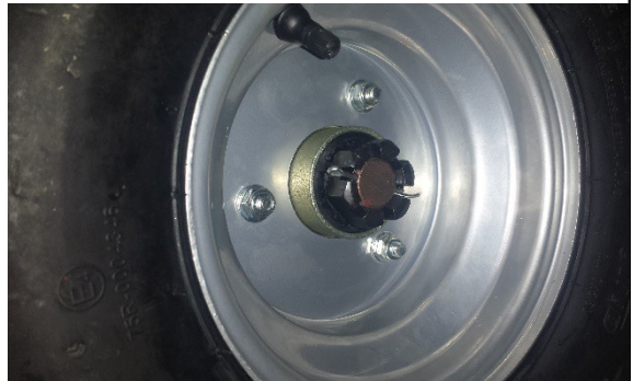
Stage 2 – fit with split pins just tight enough to get split pins in
